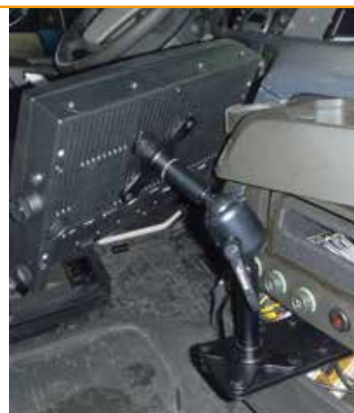
Pictured start bracket 201040-601040 Vesa 75-601051 tub 50mm-601030 Joiner Large- 601051 tub 50mm-601040 Vesa 75
