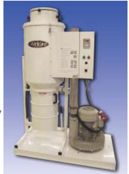
All these units have a sidechannel blower with a direct coupled 3-phase motor, and are built on compact stands. Complete unit made in epoxycoated steel. All units have low-voltage connection for remote-start from valves, and are prepared for permanent electrical power connection supply.
