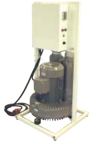
Choose between a pump-unit with a standard electrical box for 50Hz drive, or with an self-regulating speedregulator (Type "F" =inverter). All units have a vacuum relief valve as standard, to prevent overload of the pump/motor. All units supplied for permanent electrical installation.
