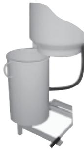
Dust are collected in an excentric supported 50L dustcan. Can fits with a plastic-bag of 100L, kept in place by vacuum in bottom of the Can. -Just move the handle down and "swing out" the dustcan! Remove the plastic bag with dust, and replace with a new.
