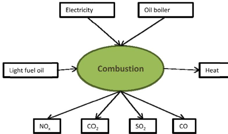
**Fig. 5: Input and emissions when the light fuel oil is combusted in an oil boiler.**
