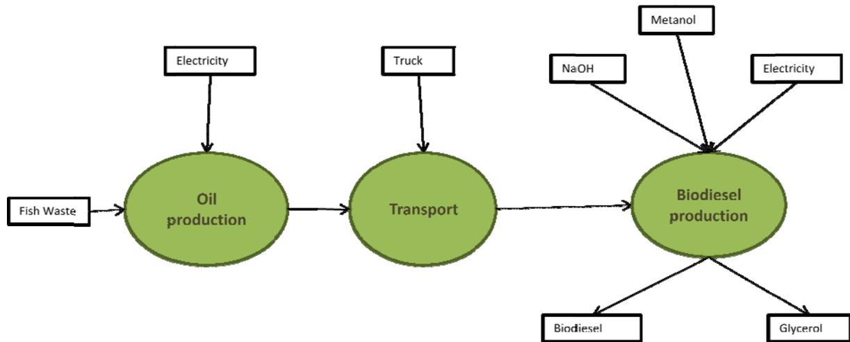
Fig. 3: The main unit processes in the fish oil scenario.
