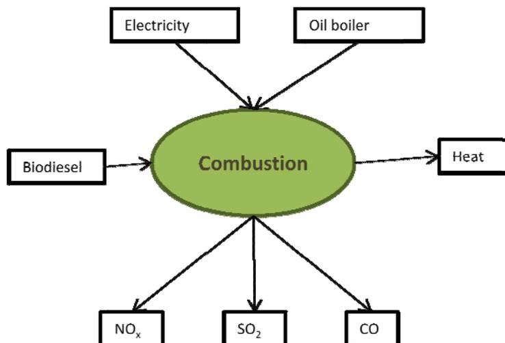
Fig. 4: Input and emissions when the biodiesel is combusted in an oil boiler.
