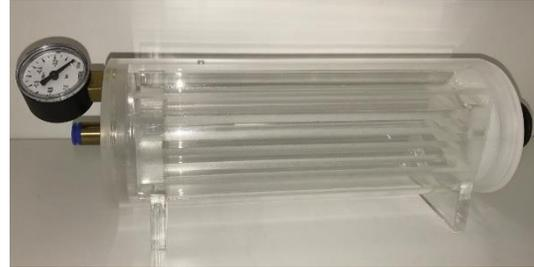
The tester consists of one or more interchangeable clamp shelf units and a minimum size vacuum container. The clamp shelf unit with integrated lid and handle is tightly fitting in the fully (360°) transparent vacuum container.
