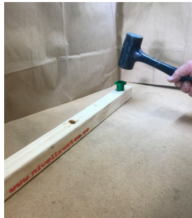
Use a rubber mallet to knock in the threaded sleeve.
