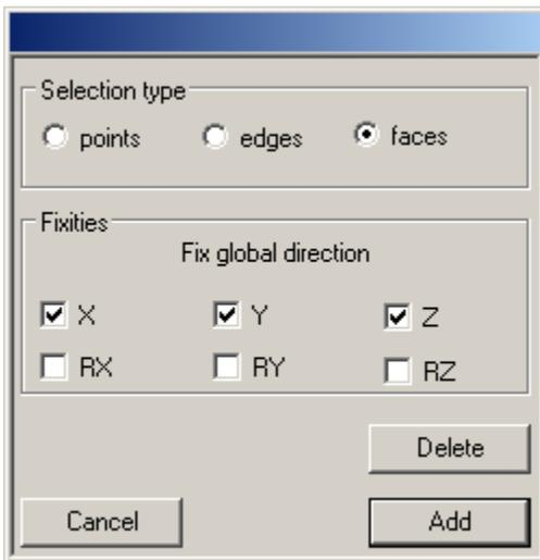
Select the 'X' 'Y' and 'Z' checkboxes under 'Fixities'. This will fix, or create a "ground" or unmovable face. More than one face can be grounded.
