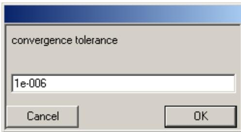
This is where you can enter the allowable error in the solution. The default, which is 0.000001, is usually sufficient.
