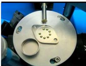
Headers with extended mounting flanges like the TO-5 can be done without loss of plating. We provide "profiled" tools with cutting areas dimensioned for your cap flange, so machined surfaces will be fully covered by the new cap. *Note: for one-shot welding, consider caps with weld projections, as the header will be machined flat during de-lid.*
