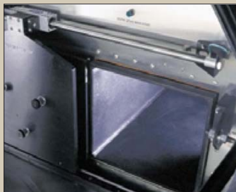
Pictured: Automatic internal sliding door
