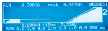
Run Screen – Constant power first pulse breaks through oxides.
