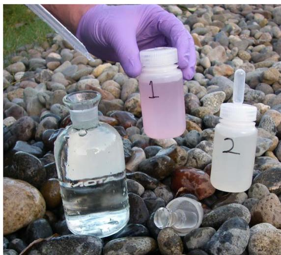
**Figure 2. Reagent containers with holes for pipette filling and storage.**
