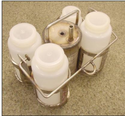
Figure 3a. APHA type DO sampler
