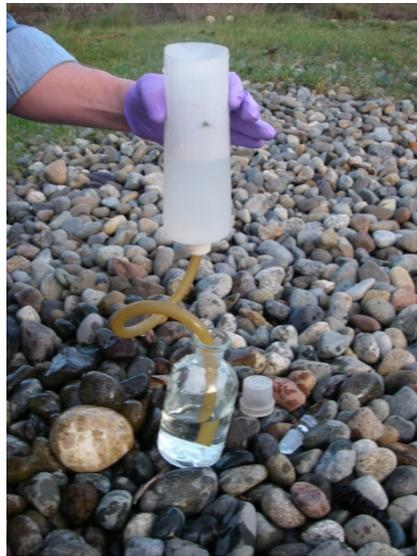
Figure 3c. Funnel-Tube surface sampler
