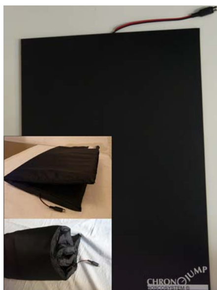
Figure 5: Main image; a photograph of the Rigid A2 platform, two inset images; photographs of the flexible platform.
