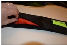
Make sure that the red string hangs freely outside the black holster so you can pull it in case of manual emergency. Check to make sure the CO2 cylinder is new and non-perforated, and that cartridges date is not expired.
