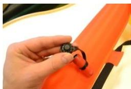
Hold and press until all air is out and the orange / yellow tube is fully deflated.
