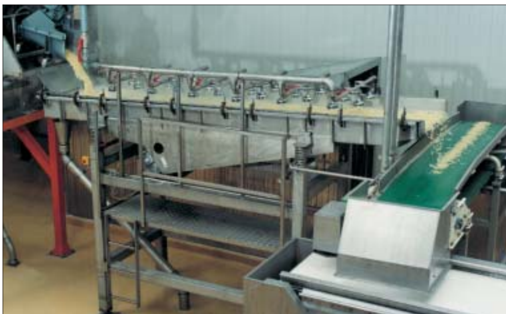
Figure 22 ESR 30/6 dewatering screening machine, 3000/600 mm, in a canning factory
