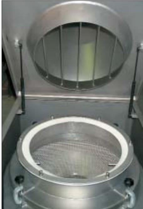
Figure 42 RS 5/4 round screening machine in a sack feeding station
