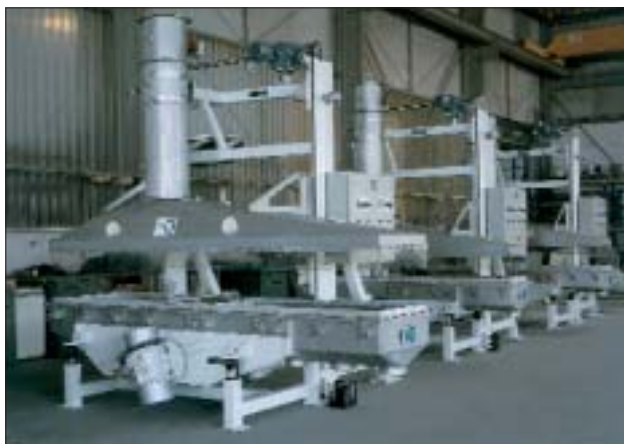
Figure 29 The guard of the fluid-bed dryer with integrated screen can be raised with the aid of a lifting unit to facilitate rapid cleaning.
