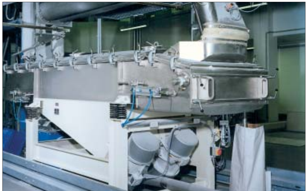
Figure 16 SR 36/10-I vibratory screening trough conveyor Screening area 3600 x 1000 mm
