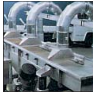
Figure 20 The dewatering effect can be considerably improved by air nozzles.
