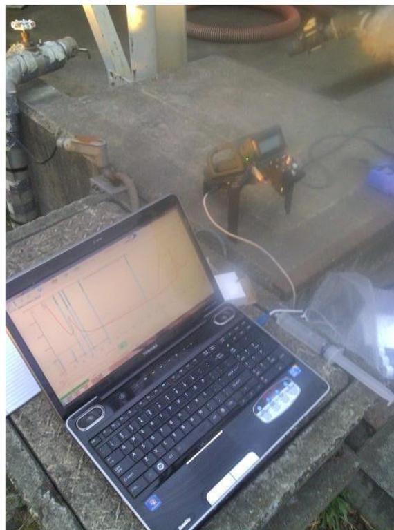
Figure 2: The FROG 4000™ is at well EW-1 analyzing water live in the field. The large syringe pictured next to the laptop is used to rinse the sparge bottle and sparge needle between samples.
