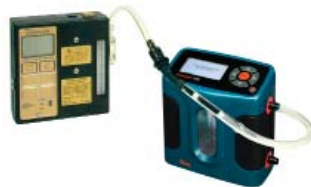
Calibration train with tube in low flow holder
