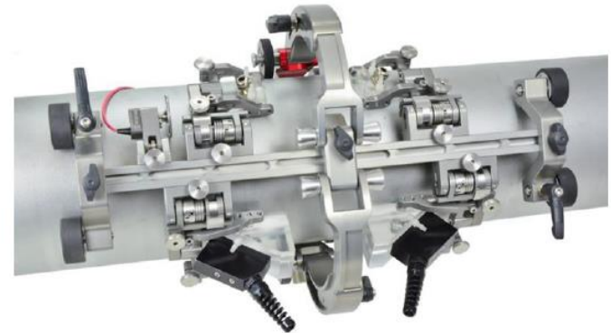
Figure 2 - Example of chain scanner with multiple probe attachment
