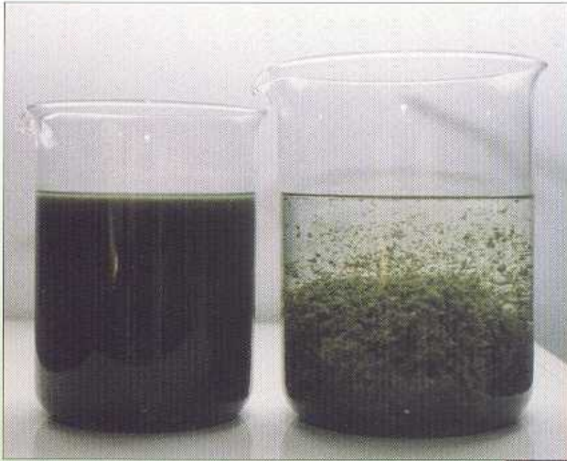
Sludge conditioning with polyelectrolyte
