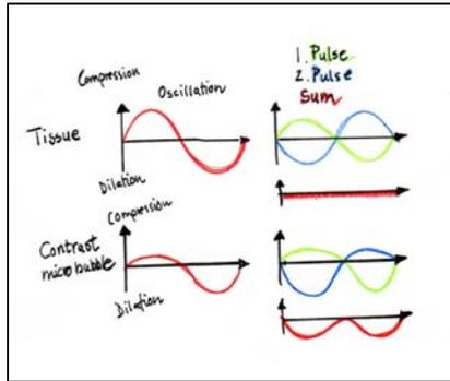
Figure 3 Summation of interpulse phase inversion sequences for linear tissue response and non-linear microbubble response.
