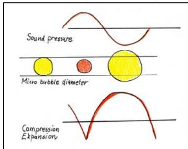
Figure 2 The nonlinear response of microbubbles to ultrasound beams. Adapted from Greis<sup>2</sup>.
