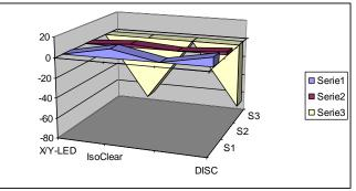
Serie 1 = Vibrations on the floor. Serie 2 = Vibrations on the Isoclear (left column). Discs of Silence equipped Radius rack (right column) Serie 3 = Reduction of vibrations in %
